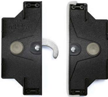
Male-Female coupling with Hook (MFG) consists of simply bringing the panels together and subsequent fixing with eccentric hooks embedded in polyurethane (variable pitch with min. 400 mm). The hooks consist of a plastic shell and a cam closing mechanism in galvanised steel.
